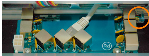
Figure 5: Power Distribution Board
