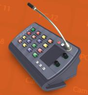
Auxiliary, rear-panel stereo analog I/O, including a studio-quality mic pre-amplifier, means that the INF-MP-16 can be used as a contribution or monitoring endpoint. The addition of GPIO as standard enables remote control of signalization or complex logic interfacing across the network infrastructure.
