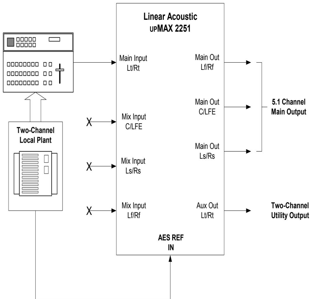
**Figure 3-1** upMAX 2251 in a commercial upmixing application
