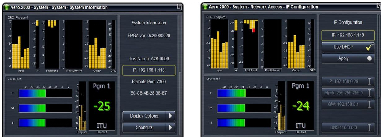
**Figure 5-3** Left: IP address, remote port, and MAC address; Right: reconfiguring IP settings
