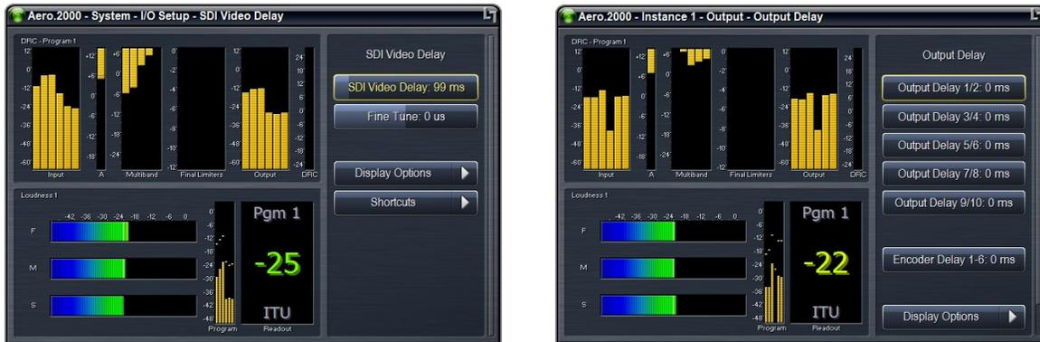
**Figure 5-5** Left: SDI video delay settings; Right: Output Delay settings available for each instance
