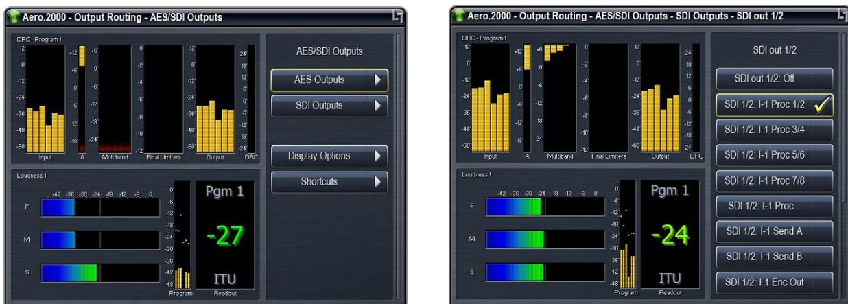
**Figure 5-4** Left: main AES outputs (BNC and DB25) and SDI outputs; Right: SDI output setup
