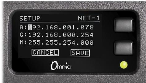
3. Press the top button on the Front Panel until the NET 1 page appears.
