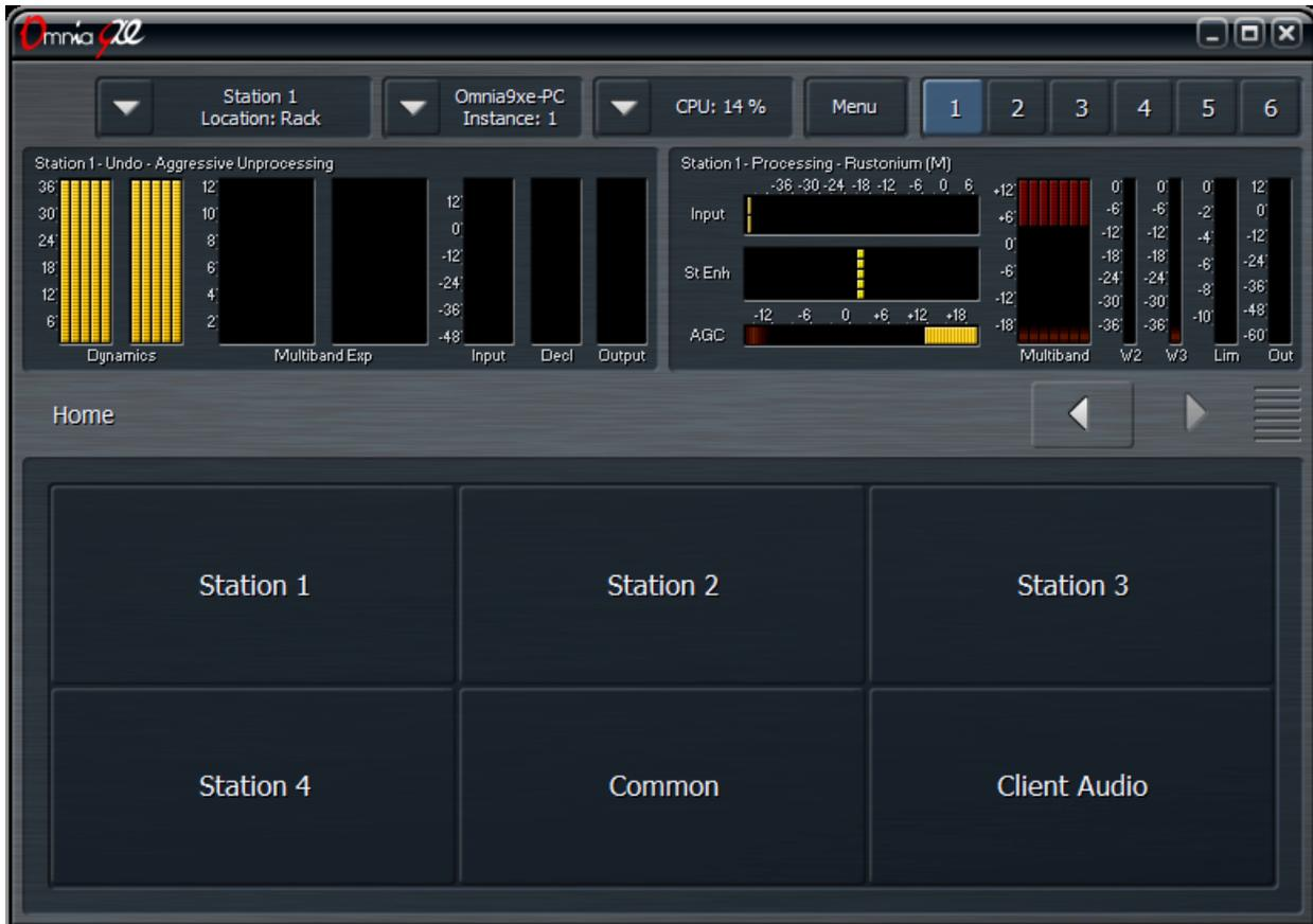
Joining the Home screen is an additional **Client Audio** menu which contains additional menus for Client Audio Output, Client Microphone Input, and Client File Recorder.
