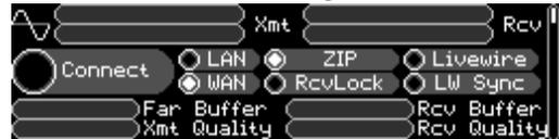
The ZIP indicator is your assurance that your Z/IP ONE is communicating with the Telos ZIP Server, and that connections to other Z/IP ONEs and Zephyr/IPs are just two button presses away.
