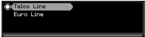
Your Z/IP ONE is factory programmed with two contacts - the Telos Line in Cleveland, Ohio, USA, and the Euro Line in Freising, Germany. Highlight "Telos Line" and press the AUTO button again (or push the main control knob) to establish a call. As the call progresses and connects, the screen changes automatically to the main Status display.
