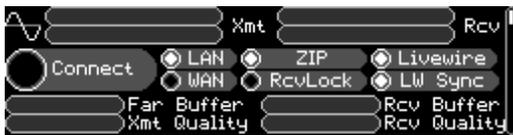
The first screen displays broad information on a number of systems. At the top of the display are level meters for the transmitted and received (decoded) audio. The left channel is at the top, with the right channel under it. To the left of the meters is an indicator of what audio input is currently being used. This is especially useful when input failover is enabled. The icons have the following meanings:
