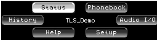
Turning the Z/IP ONE's control knob will move the highlight between these options. The name shown in the middle of this screen is the device's identity on the ZIP Server, used for making calls without having to memorize IP addresses.
