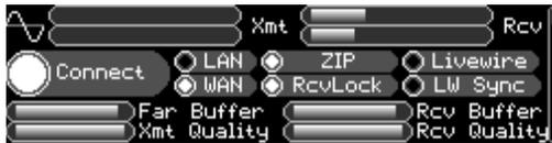
The large *Connect* indicator should come ON quickly, followed a few seconds later by the *RcvLock* indicator. The *Rcv* audio level meters will begin showing moving audio levels. In a few more seconds the *Buffer* and *Quality* gauges in the lower third of the screen will show relative indications of receive buffer size at both ends and quality of the connection, indicating dropped packets.
