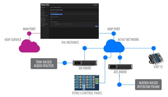
The diagram above shows an example system with a non-AoIP mixer and intercom system using a Telos Alliance AES xNode and SDI Node.
